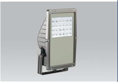
The AMELIA LED FLOODLIGHT is a general purpose asymmetric floodlight designed to meet the requirements of commercial and industrial floodlighting. A die cast aluminium housing and frame incorporates 5mm thick tempered glass and wide cooling fins produces excellent temperature control. Excellent resistance to corrosive and saline environments is achieved with a polyester powder coated silver finish.
